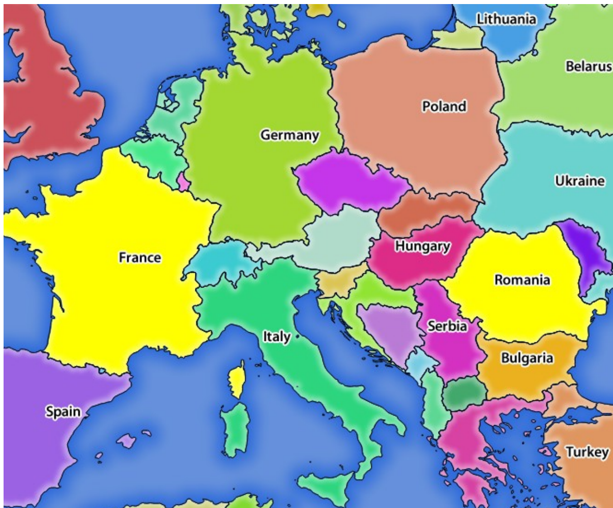
Fig. 3.4: Server response to a GetMap request with SELECTION parameter
