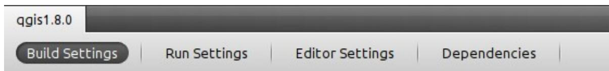
We now want to add a custom process step. Why? Because QGIS can currently only run from an install directory, not its build directory, so we need to ensure that it is installed whenever we build it. Under 'Build Steps', click on the 'Add BuildStep' combo button and choose 'Custom Process Step'.
