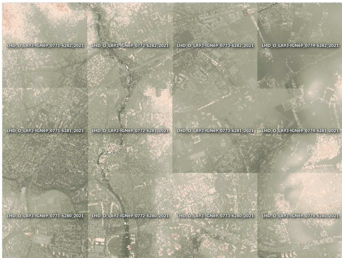
Fig. 16.15: Individual point cloud tiles loaded, with artefacts on edges
