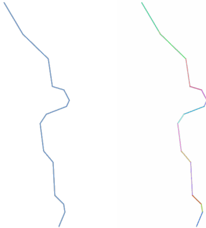
Fig. 24.84: The original line layer and the exploded one
