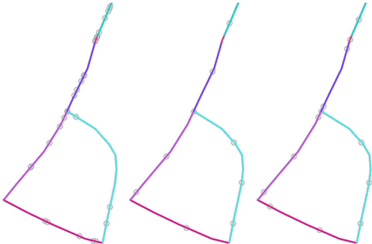
Fig. 24.55: Five points per line feature, left : min. distances = 0, middle : min.distances != 0, right : min. distance != 0, global min. distance = 0
