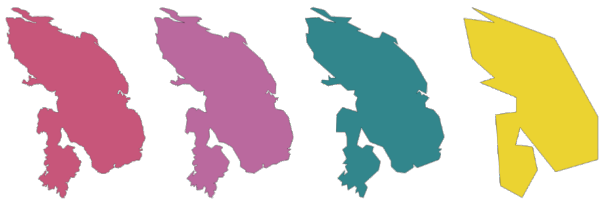
Fig. 9.28: From left to right, source layer and increasing simplification tolerances
