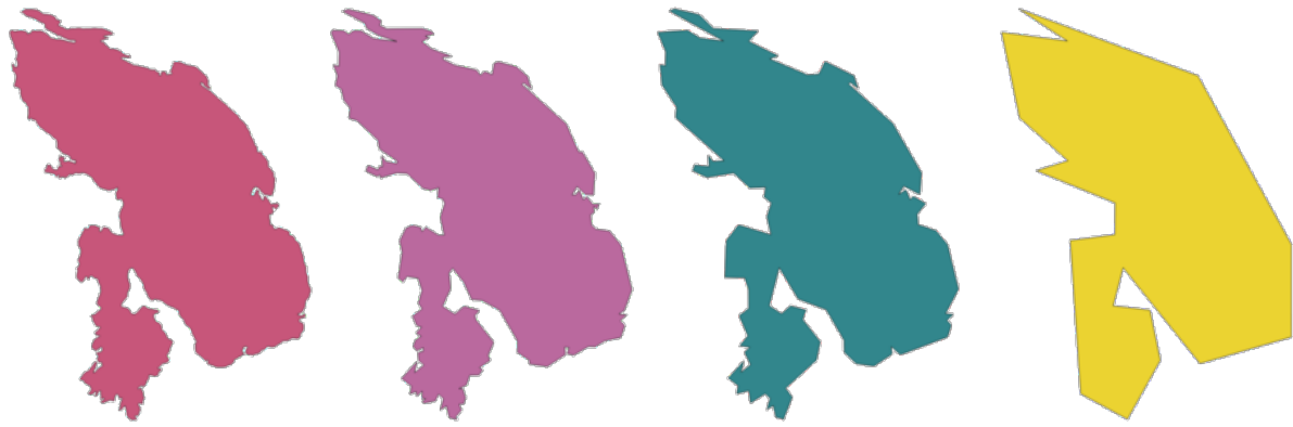
Fig. 24.107: From left to right, source layer and increasing simplification tolerances
