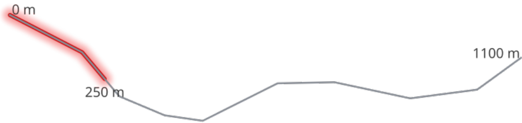
Fig. 24.91: Substring line with starting distance set at 0 meters and the ending distance at 250 meters.
