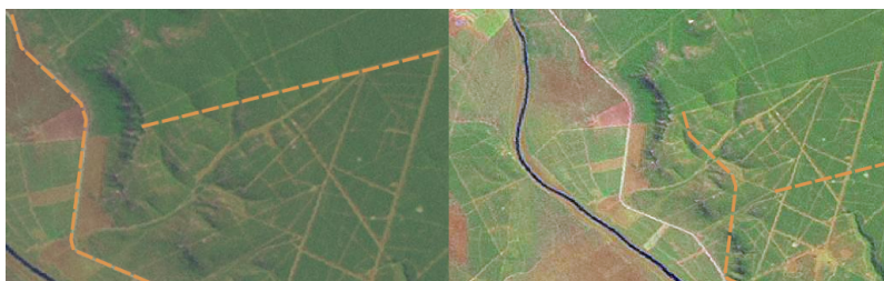
Слика5.9: The importance of using properly georeferenced raster images for heads-up digitising. On the left we can see the image is properly georegistered and the road features (in orange) overlap perfectly. If the image is poorly georeferenced (as shown on the right) the features will not be well aligned. Worse still, if the image on the right is used as a reference when capturing new features, the newly captured data will be inaccurate!
