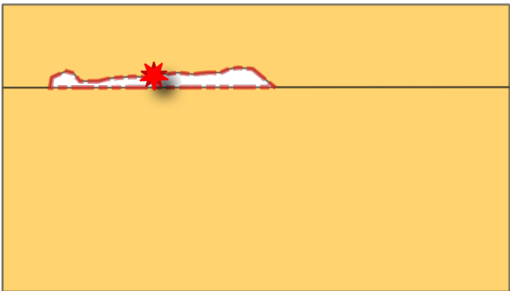
Fig. 24.14: Reporting errors on polygon features for gaps smaller than the specified threshold.
