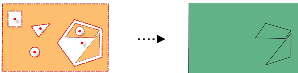
Fig. 24.21: Deleting holes in a polygon feature.
