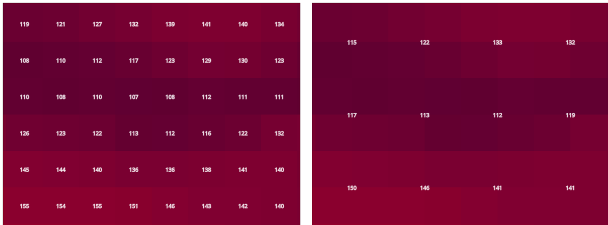
Fig. 13.15: Pixels labeled using various resampling options
