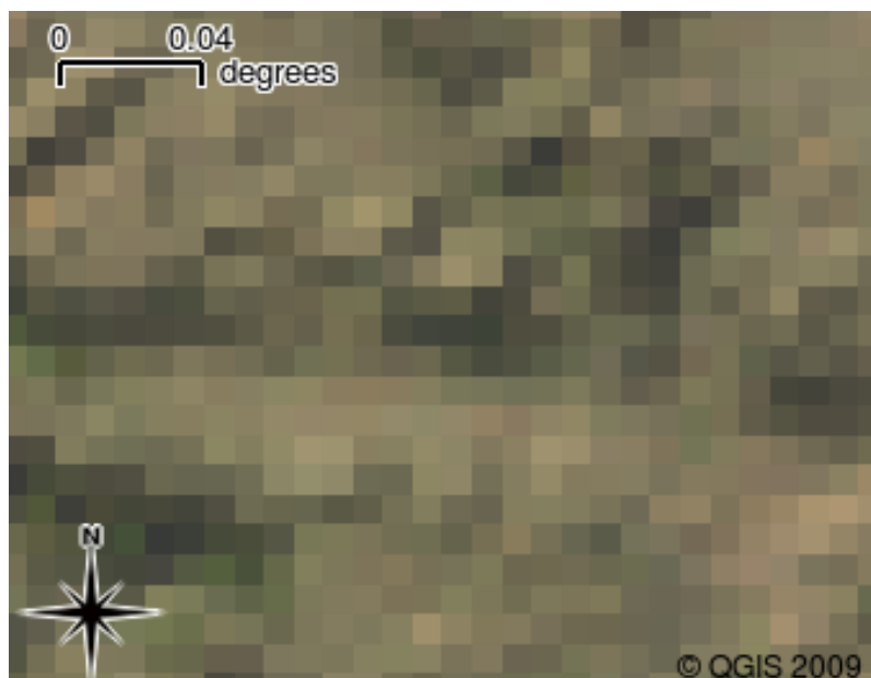
Rys. 2.13: The same raster data, but this time zoomed in. The grid nature of the data can be seen.
