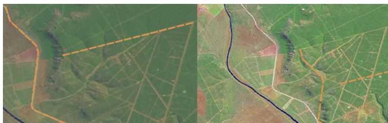
5.9 Fig. : The importance of using properly georeferenced raster images for heads-up digitising. On the left we can see the image is properly georegistered and the road features (in orange) overlap perfectly. If the image is poorly georeferenced (as shown on the right) the features will not be well aligned. Worse still, if the image on the right is used as a reference when capturing new features, the newly captured data will be inaccurate!
