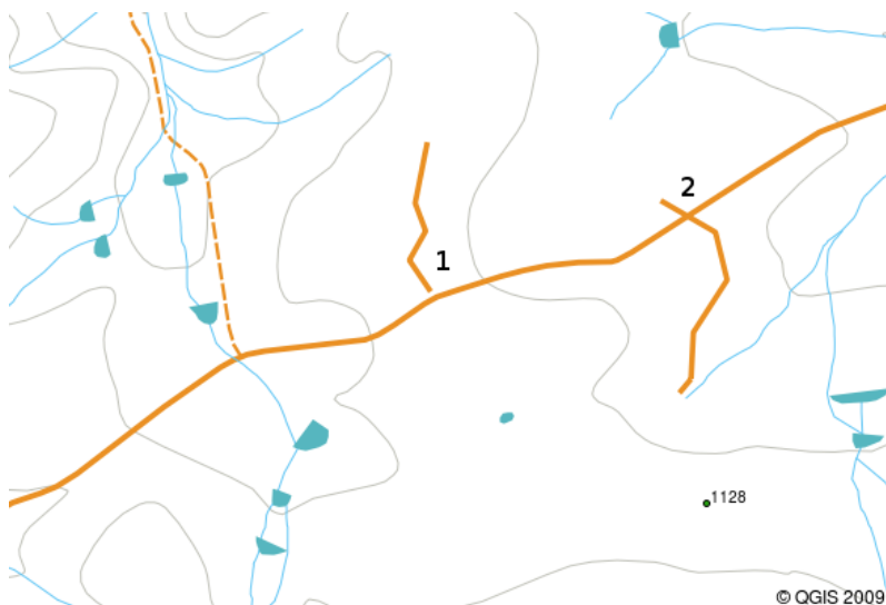
Fig. 3.13: Undershoots (1) occur when digitised vector lines that should connect to each other don't quite touch. Overshoots (2) happen if a line ends beyond the line it should connect to.
