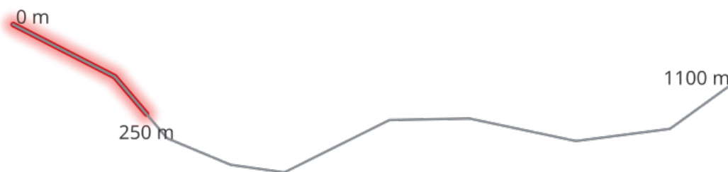
Fig. 9.19: Substring line with starting distance set at 0 meters and the ending distance at 250 meters.
