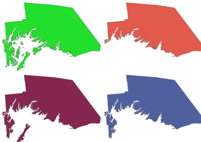
Fig. 28.88: Clockwise from top left: original multipart feature, one, two and three biggest parts kept
