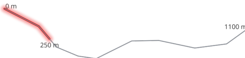
Fig. 13.19: Substring line with starting distance set at 0 meters and the ending distance at 250 meters.
