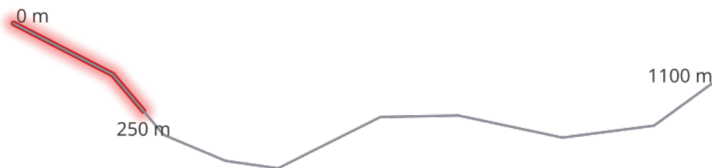
Fig. 28.89: Substring line with starting distance set at 0 meters and the ending distance at 250 meters.
