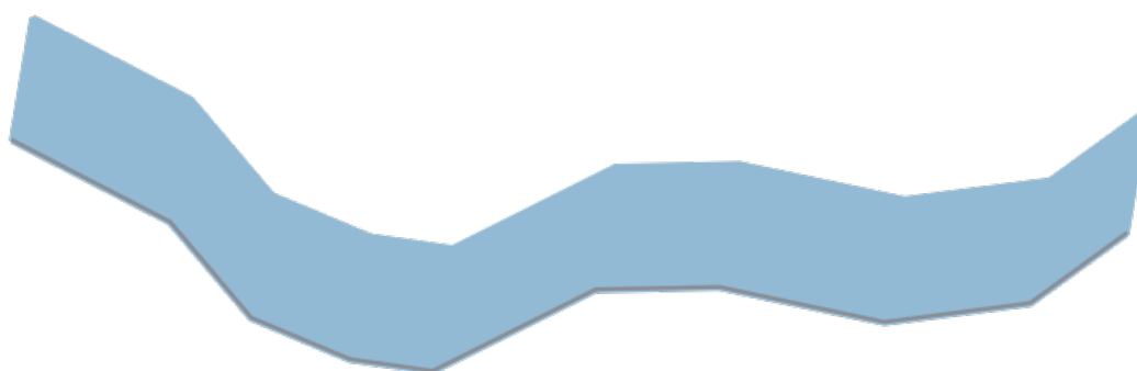
Fig. 13.17: Generating a polygon by extruding a line with offset in x and y directions
