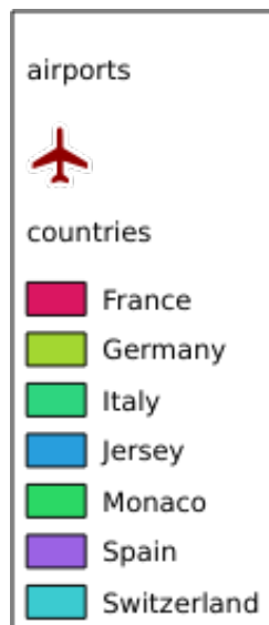
Abb. 3.5: Legend rendering without label for single symbol layers
