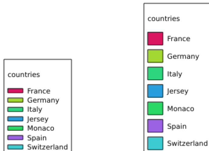
图 3.12: To the left SYMBOLHEIGHT=2 and to the right SYMBOLHEIGHT=6
