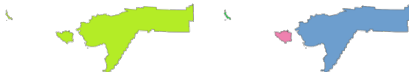
Fig. 28.93: Left the multipart source layer and right the single part output result
