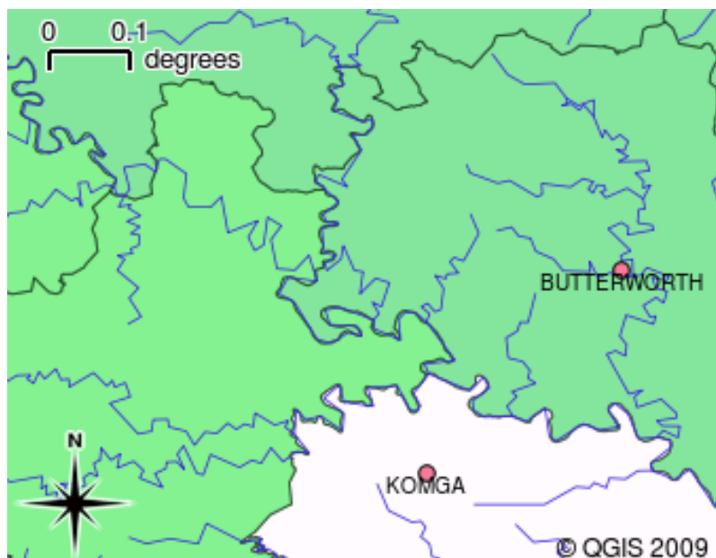
Fig. 2.11: Vector data is used to represent points (e.g. towns), lines (e.g. rivers) and polygons (e.g. municipal boundaries).
