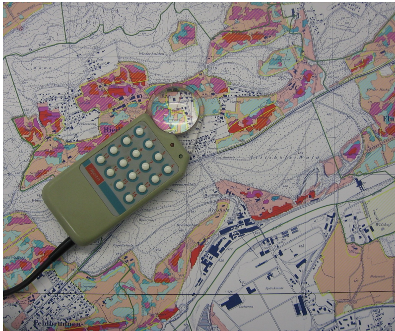
Abb. 5.8: A digitising table and puck are used by GIS professionals when they want to digitise features from existing maps.
