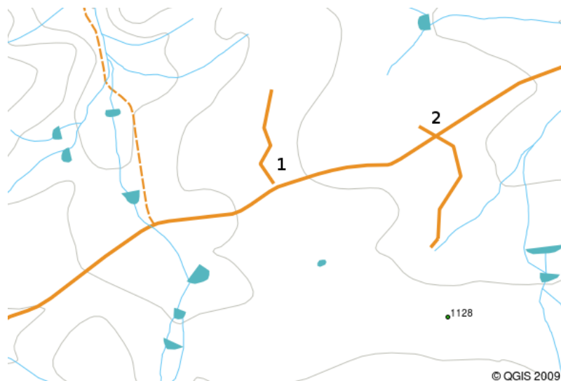
Abb. 3.13: Undershoots (1) occur when digitised vector lines that should connect to each other don't quite touch. Overshoots (2) happen if a line ends beyond the line it should connect to.
