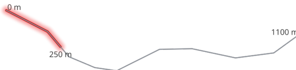
Obr. 28.89: Substring line with starting distance set at 0 meters and the ending distance at 250 meters.
