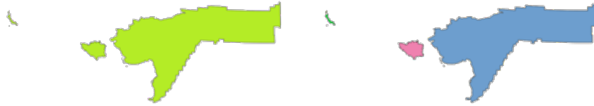
Obr. 28.93: Left the multipart source layer and right the single part output result
