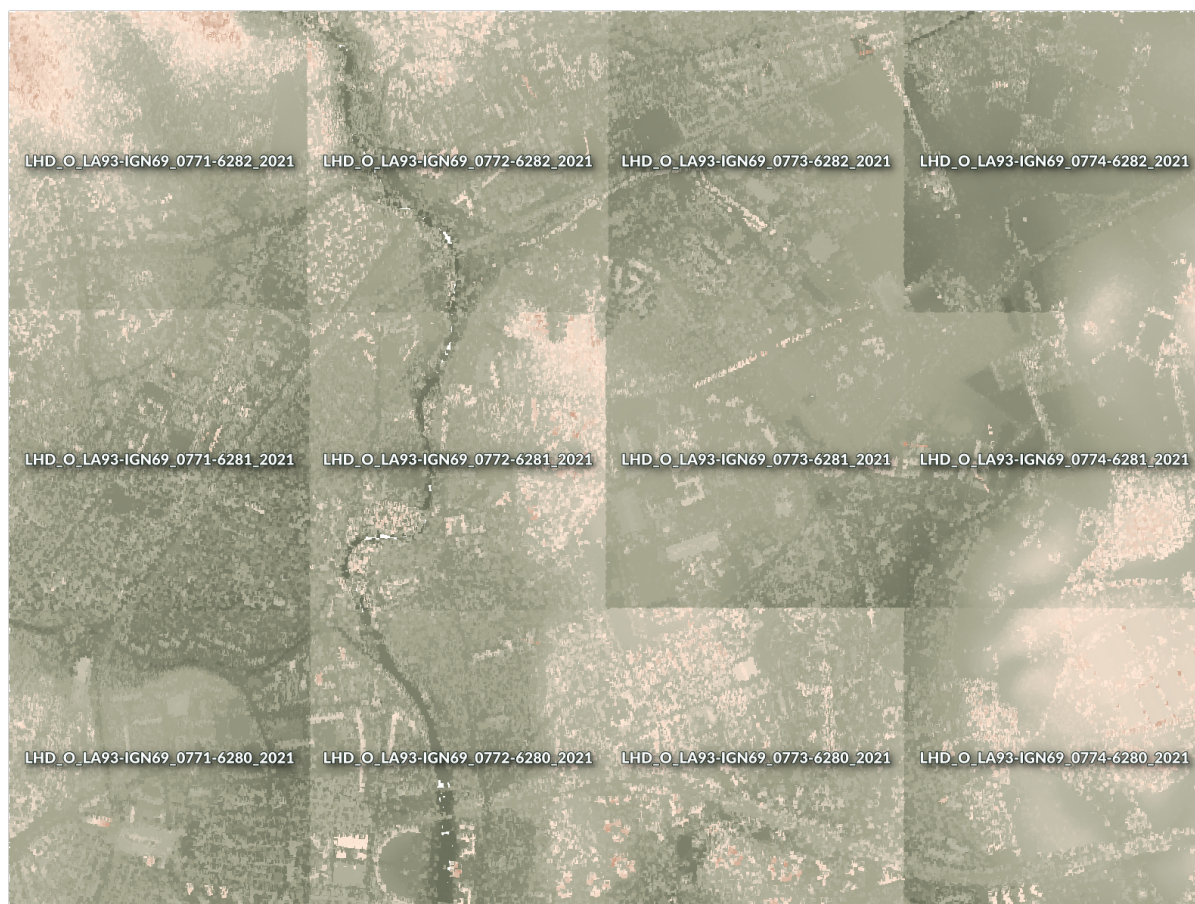
Obr. 20.12: Individual point cloud tiles loaded, with artefacts on edges
