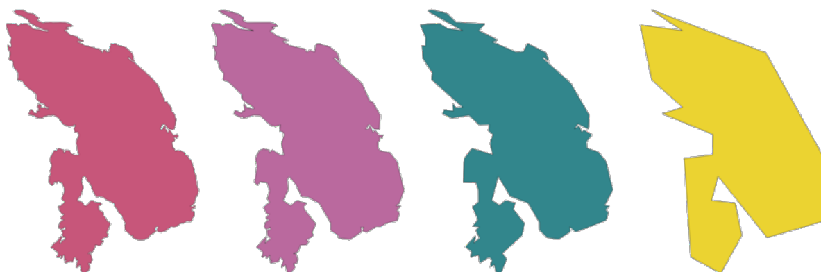
Obr. 28.105: Clockwise from top left: source layer and increasing simplification tolerances
