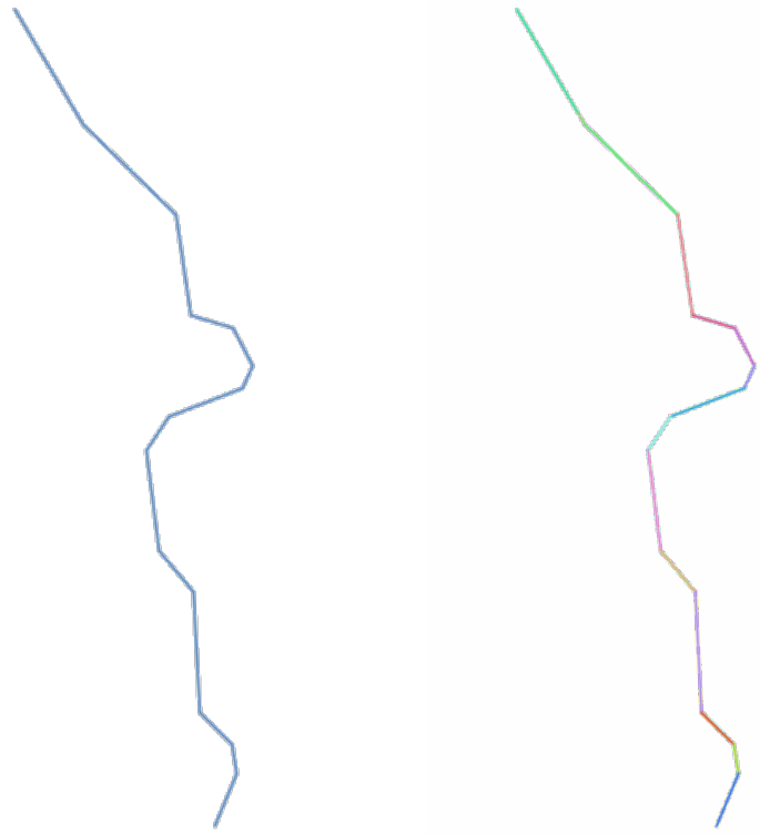
Obr. 28.82: The original line layer and the exploded one
