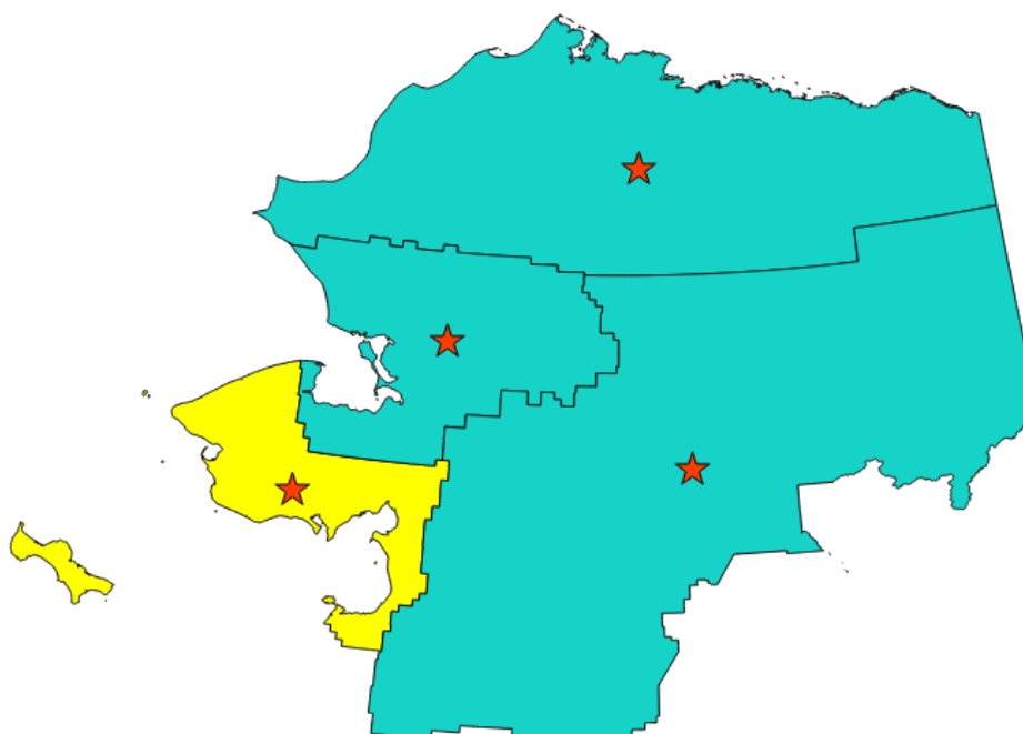
Obr. 28.68: The red stars represent the centroids of the features of the input layer.
