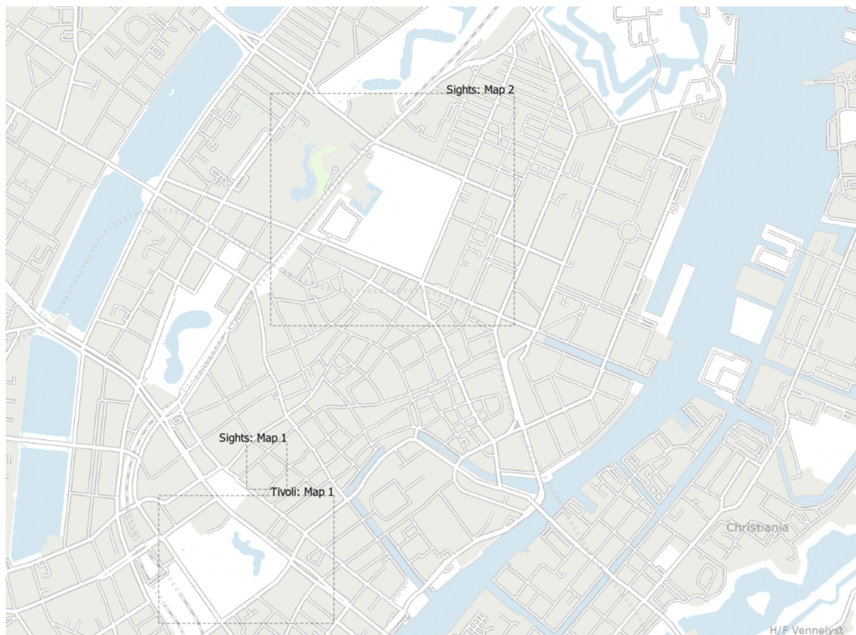
Fig. 11.11: Example of layout extents displayed in a QGIS project with two print layouts. The print layout named «Sights» contains two map items, while the other print layout contains one map item.
