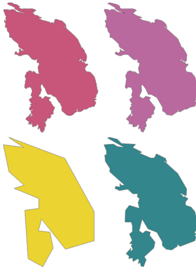
Figura27.96: Clockwise from top left: source layer and increasing simplification tolerances
