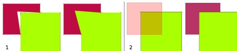
Figura7.3: (1) Topological editing to detect shared boundaries, when moving vertices. When moving a vertex, all features that share that vertex are updated. (2) To avoid polygon overlaps, when a new polygon is digitised (shown in red) it is clipped to avoid overlapping neighbouring areas.
