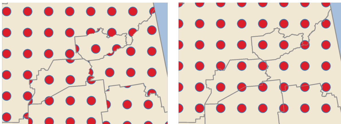
14.18 Fig. : Aligning point pattern to feature (left) and to map extent (right)
