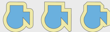
27.98 Fig. : Round, miter, and bevel join styles
