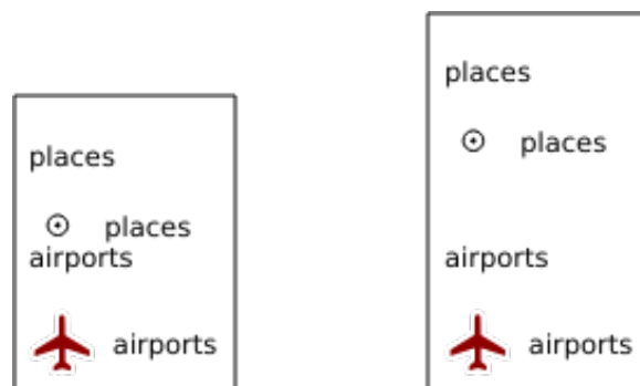
Fig. 3.7: To the left LAYERSPACE=0 and to the right LAYERSPACE=10
