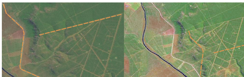
Fig. 5.9: The importance of using properly georeferenced raster images for heads-up digitising. On the left we can see the image is properly georegistered and the road features (in orange) overlap perfectly. If the image is poorly georeferenced (as shown on the right) the features will not be well aligned. Worse still, if the image on the right is used as a reference when capturing new features, the newly captured data will be inaccurate!
