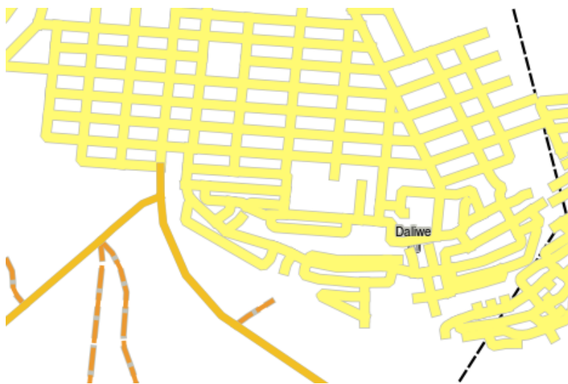
Fig. 4.14: A roads vector layer symbolised using a unique value per road type.
