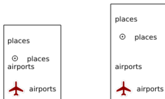
Obr. 3.7: To the left LAYERSPACE=0 and to the right LAYERSPACE=10
