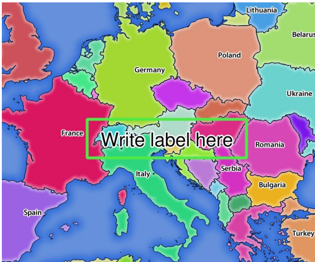
Obr. 3.21: Server response to a GetMap request with redlining parameters
