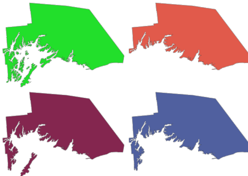
Obr. 27.79: Clockwise from top left: original multipart feature, one, two and three biggest parts kept
