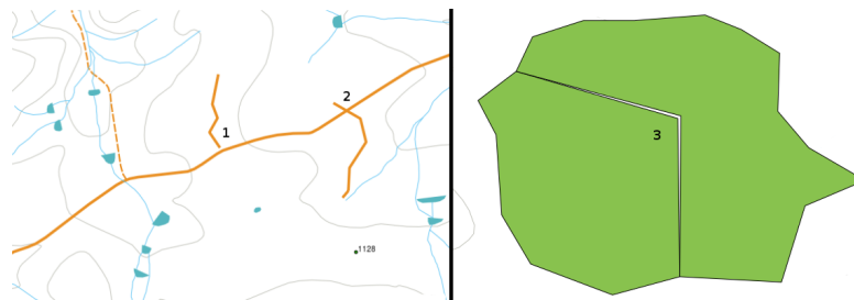
7.2 Fig. : Undershoots (1) occur when digitised vector lines that should connect to each other don't quite touch. Overshoots (2) happen if a line ends beyond the line it should connect to. Slivers (3) occur when the vertices of two polygons do not match up on their borders.
