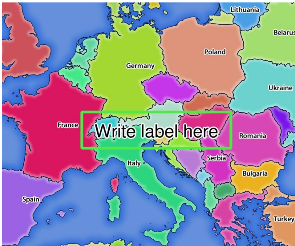
Abb. 3.21: Server response to a GetMap request with redlining parameters
