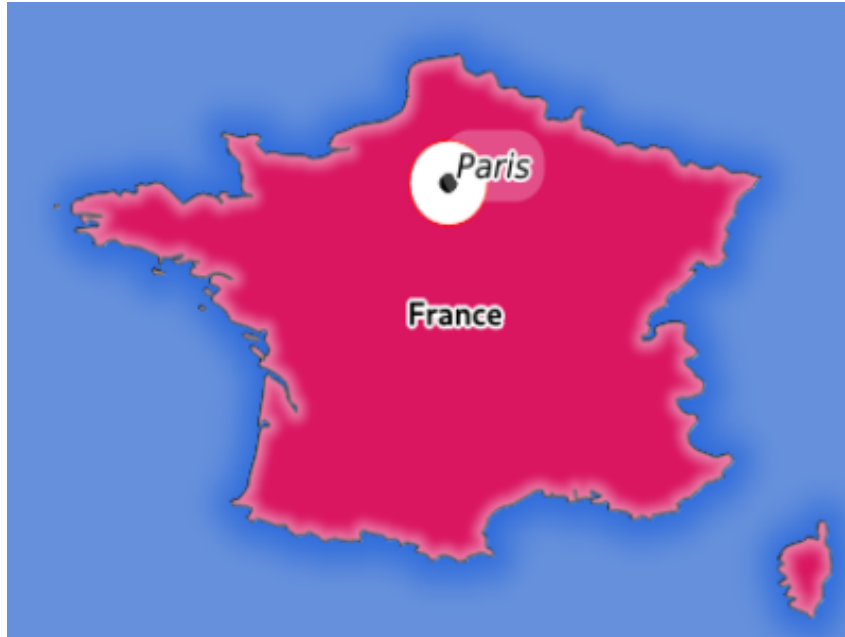
Abb. 3.3: Server response to a GetMap request with FILTER parameter
