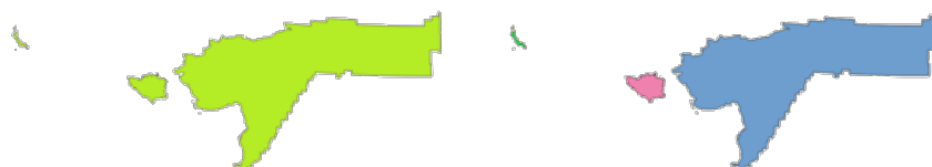
Obr. 25.78: Left the multipart source layer and right the single part output result
