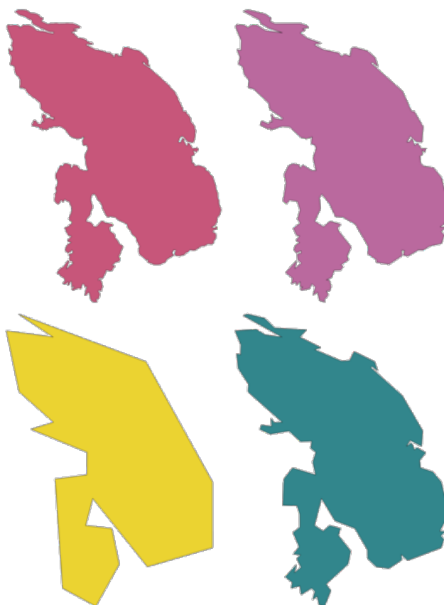
Obr. 25.89: Clockwise from top left: source layer and increasing simplification tolerances
