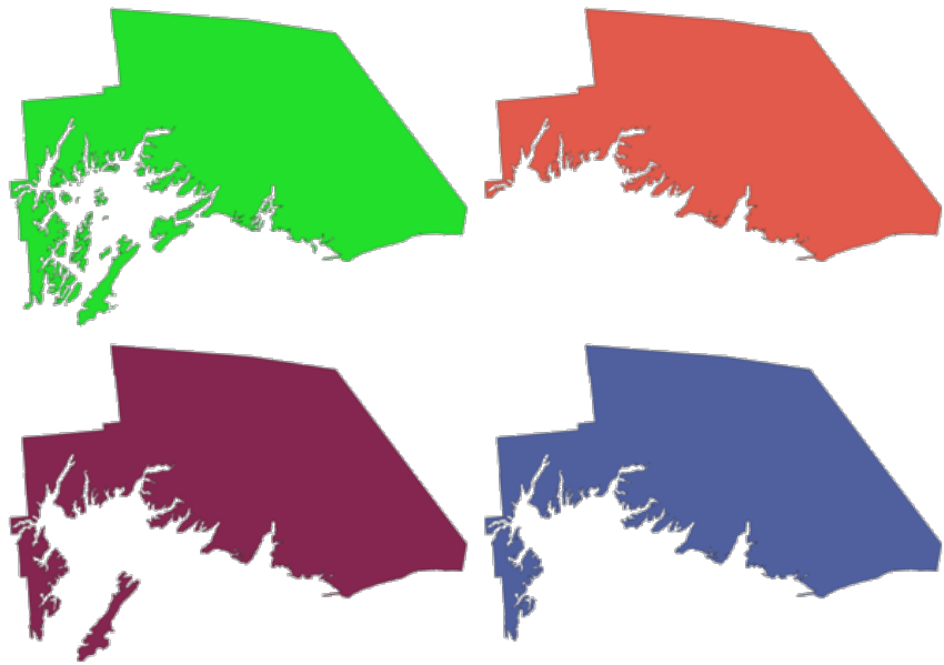
Obr. 25.73: Clockwise from top left: original multipart feature, one, two and three biggest parts kept
