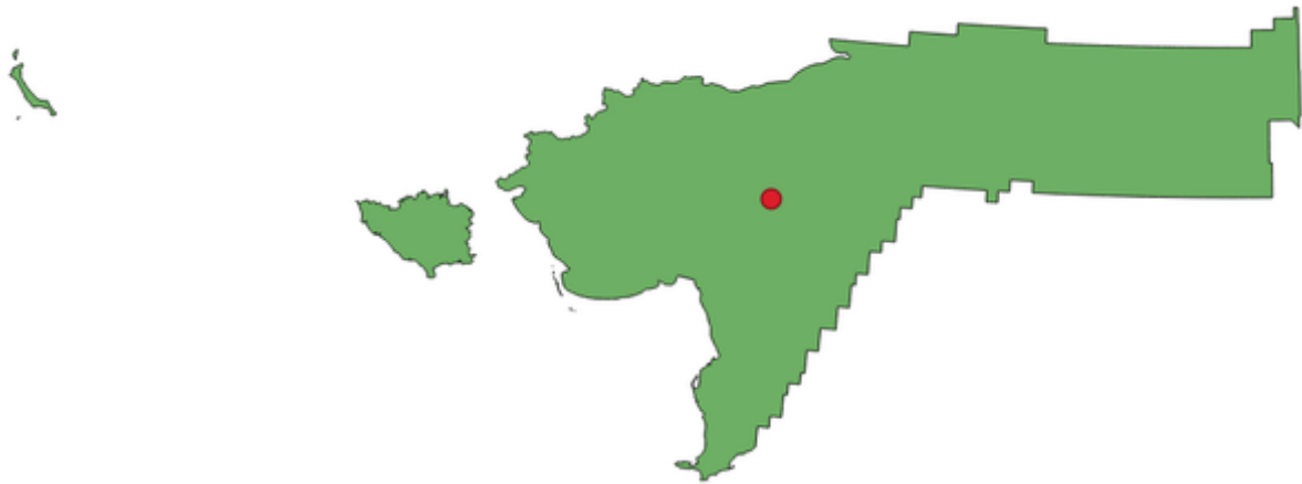
图 24.74: Pole of inaccessibility
