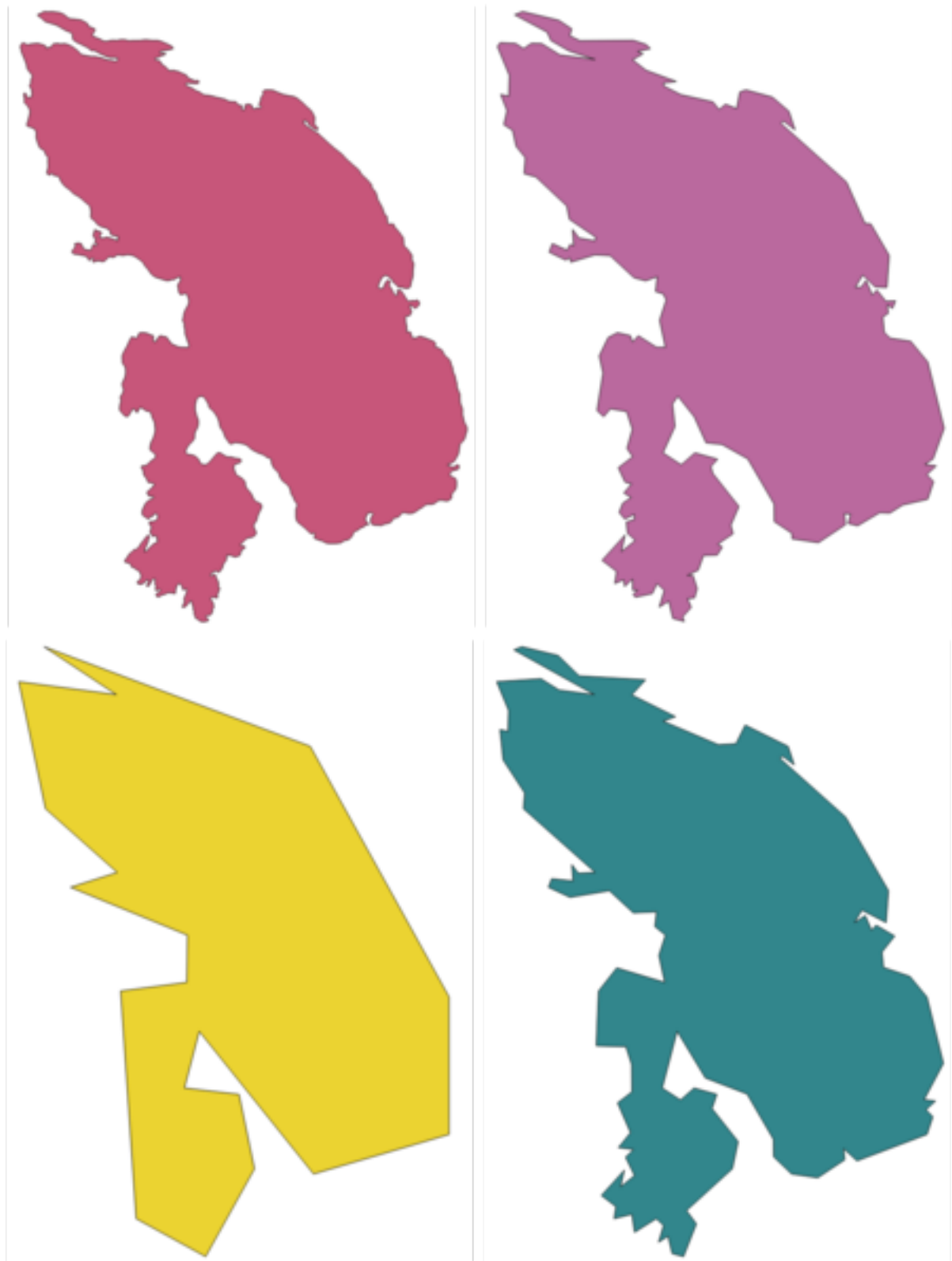
图 24.79: Clockwise from top left: source layer and increasing simplification tolerances
