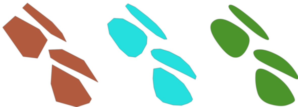
图 24.81: Increasing number of iterations causes smoother geometries
