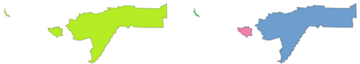
图 24.69: Left the multipart source layer and right the single part output result
