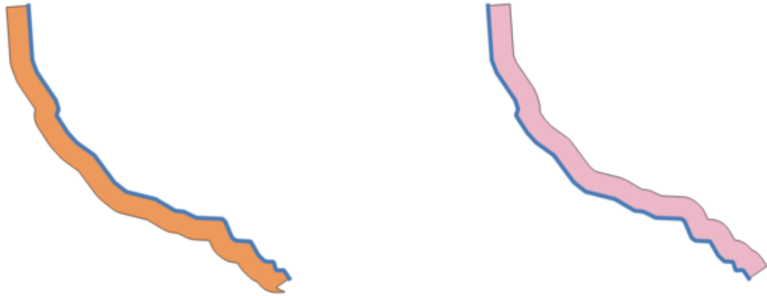
图 24.80: Left versus right side buffer on the same vector line layer
