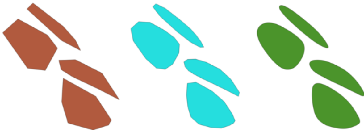
图 24.81: Increasing number of iterations causes smoother geometries
