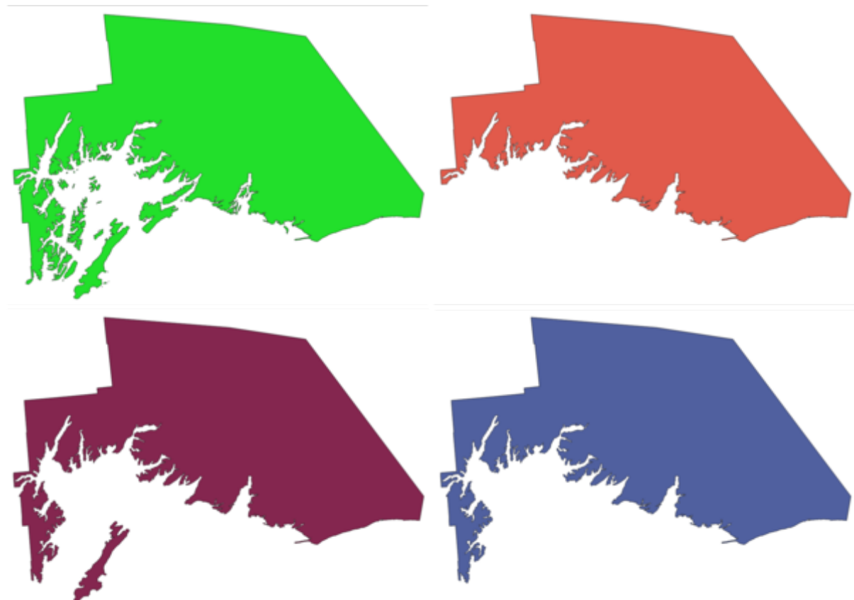
Gambar24.64: Clockwise from top left: original multipart feature, one, two and three biggest parts kept
