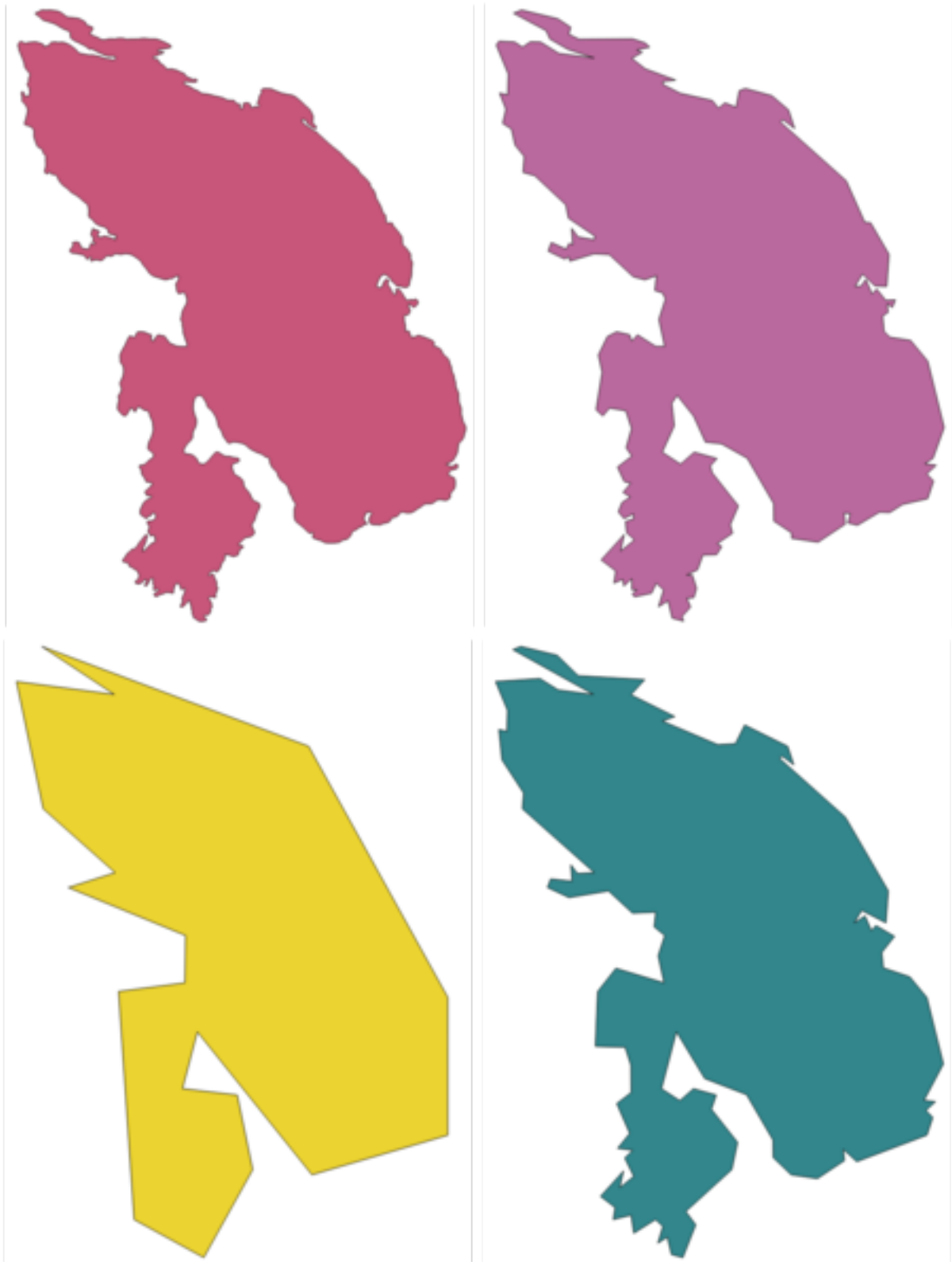
Gambar24.79: Clockwise from top left: source layer and increasing simplification tolerances
