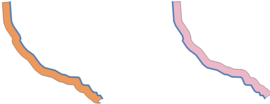
Gambar24.80: Left versus right side buffer on the same vector line layer
