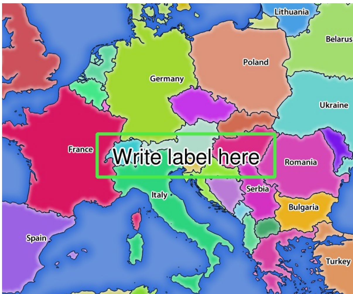
Fig. 3.7: Server response to a GetMap request with redlining parameters
