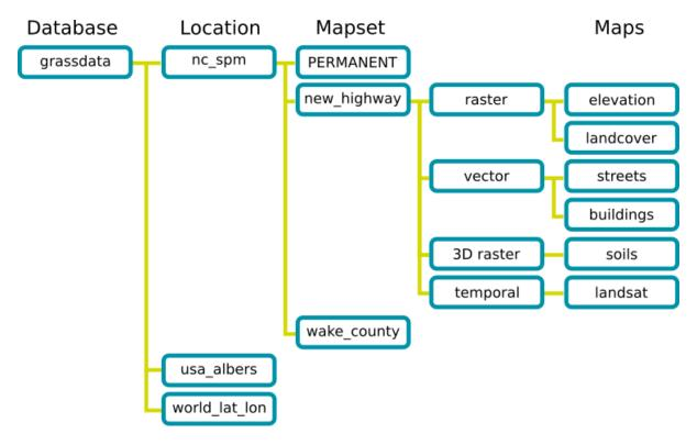
Obr. 12.3: GRASS database structure (from GRASS docs)
