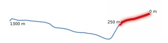
Obr. 24.65: Substring line with starting distance set at 0 meters and the ending distance at 250 meters.
