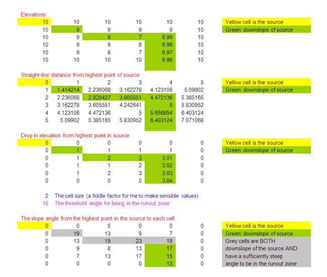
Slope is to be measured using the straight line distance from source point to evaluation point.
