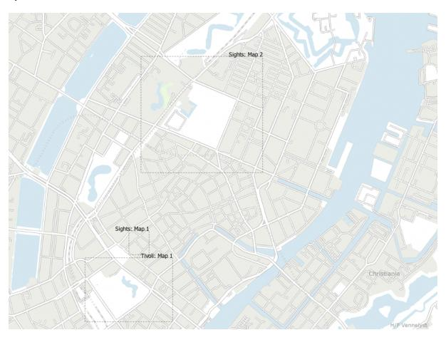
Obr. 11.13: Example of layout extents displayed in a QGIS project with two print layouts. The print layout named ,Sights' contains two map items, while the other print layout contains one map item.
