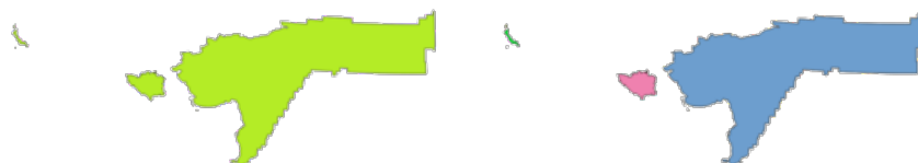
图 28.93: Left the multipart source layer and right the single part output result
