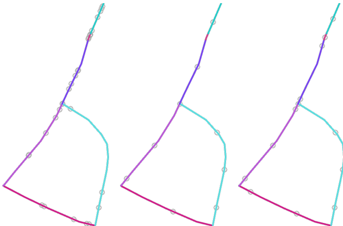
图 28.53: Five points per line feature, left : min. distances = 0, middle : min.distances != 0, right : min. distance != 0, global min. distance = 0
