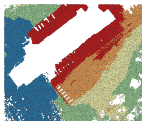
图 28.12: Exporting point cloud (ground points) to a vector layer styled based on the elevation
