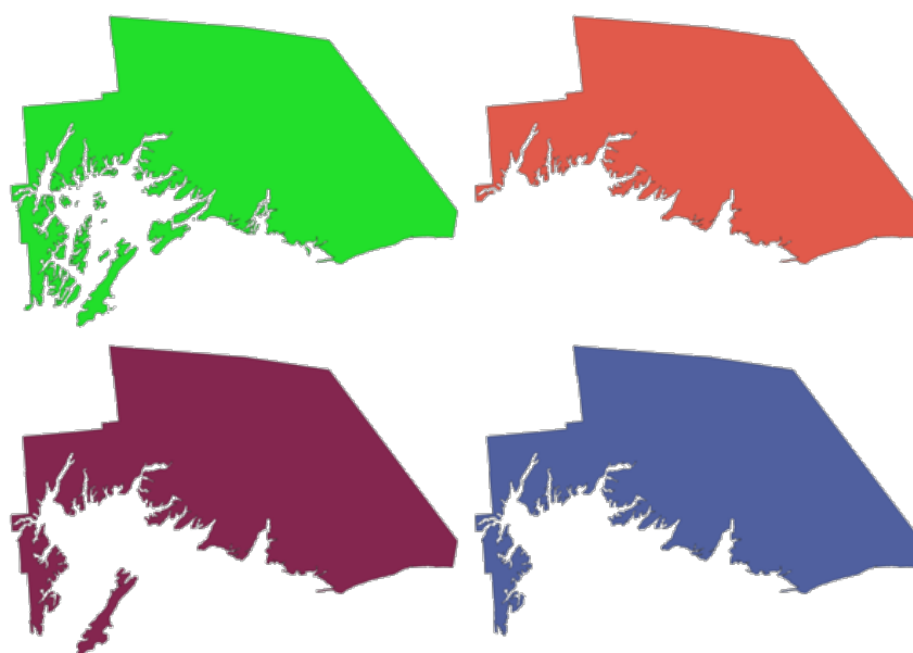
28.88 Fig. : Clockwise from top left: original multipart feature, one, two and three biggest parts kept
