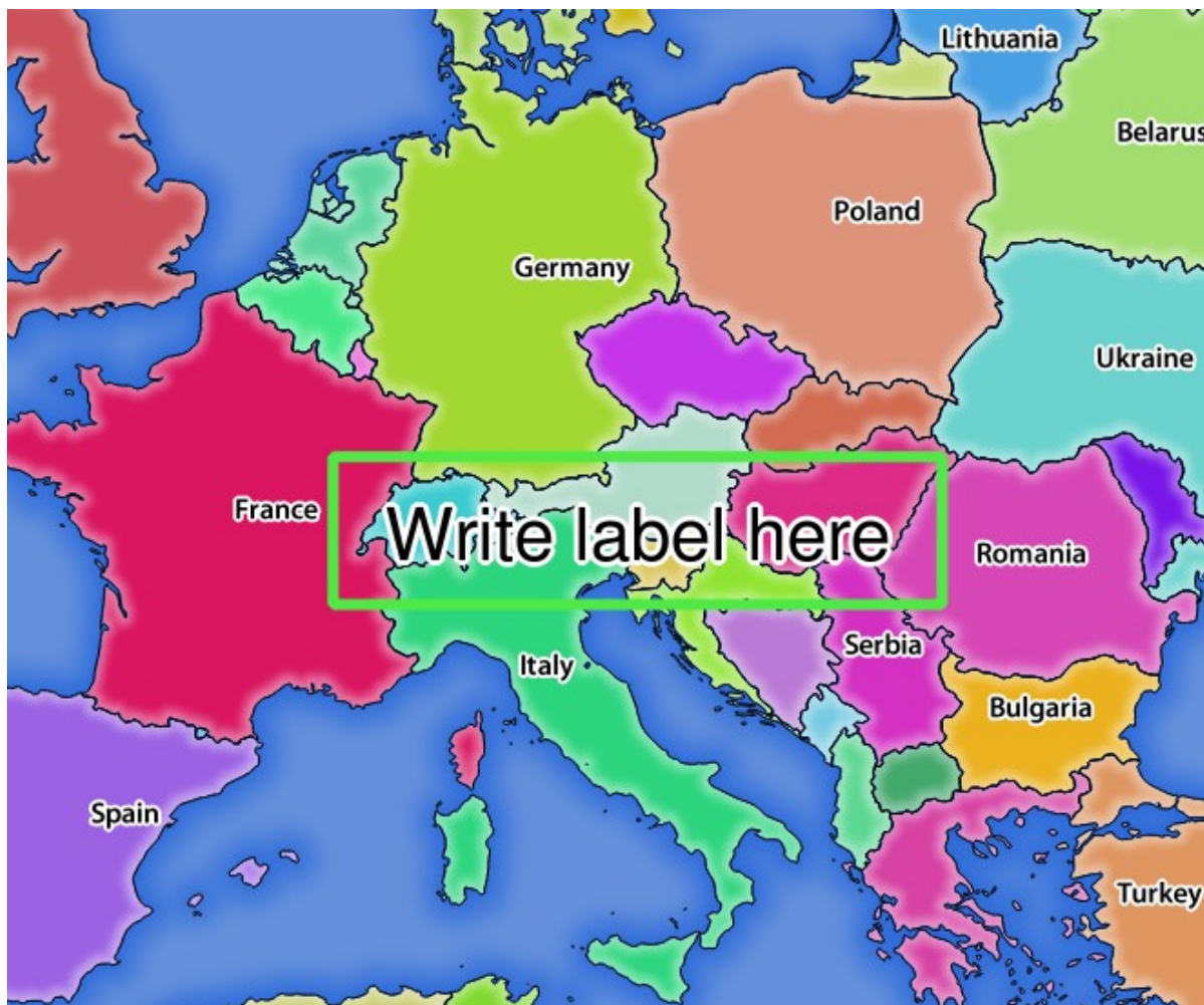
3.22. ábra: Server response to a GetMap request with redlining parameters
