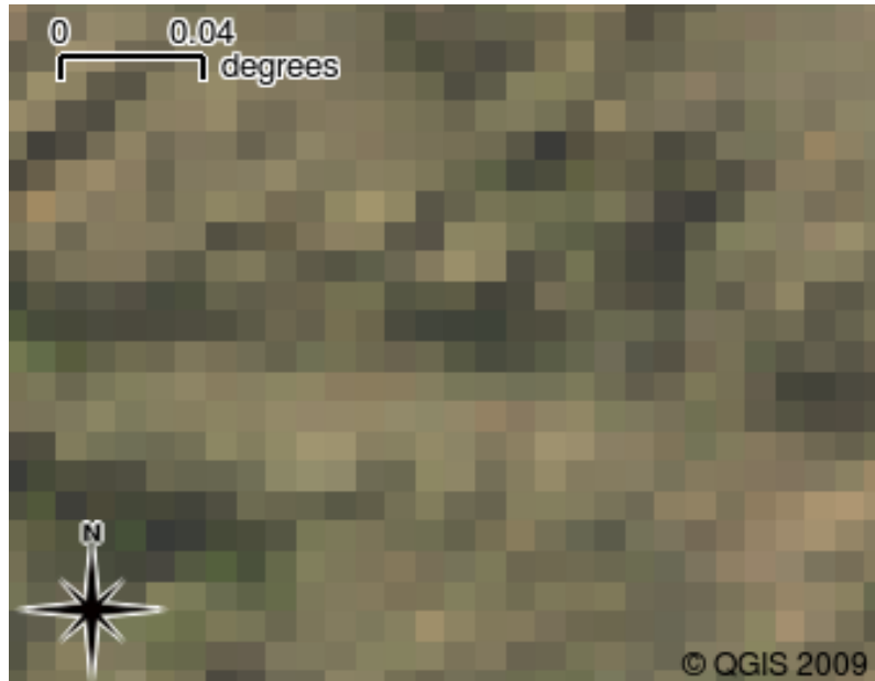
2.13. ábra: The same raster data, but this time zoomed in. The grid nature of the data can be seen.
