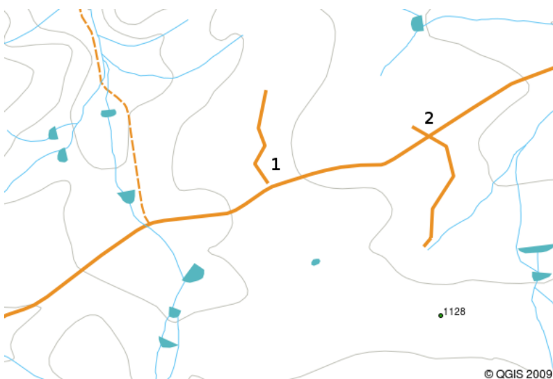
3.13. ábra: Undershoots (1) occur when digitised vector lines that should connect to each other don't quite touch. Overshoots (2) happen if a line ends beyond the line it should connect to.
