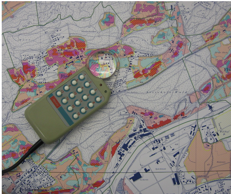
Fig. 5.8: A digitising table and puck are used by GIS professionals when they want to digitise features from existing maps.
