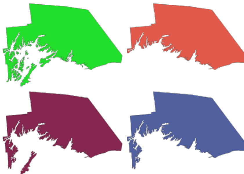
Fig. 27.88: Clockwise from top left: original multipart feature, one, two and three biggest parts kept
