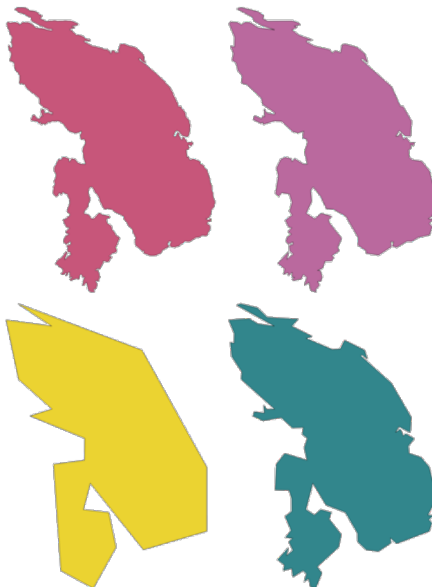
Obr. 28.105: Clockwise from top left: source layer and increasing simplification tolerances
