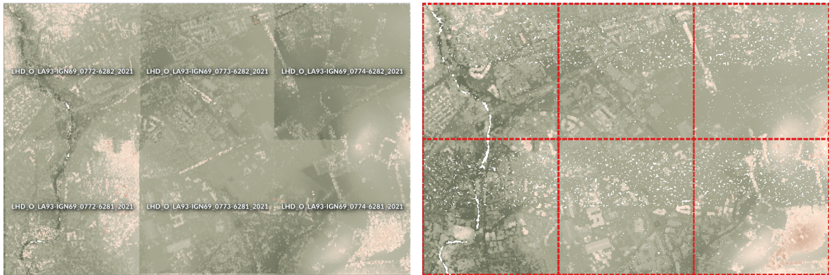
Obr. 28.13: Generating Virtual Point Cloud with overview from a set of point cloud tiles
