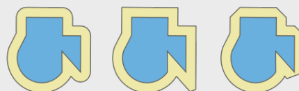
Obr. 28.107: Round, miter, and bevel join styles
