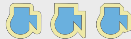
Obr. 28.64: Round, miter, and bevel join styles
