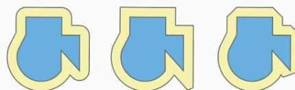
Figure28.95: Round, miter, and bevel join styles
