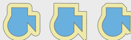
Рис. 28.107: Round, miter, and bevel join styles
