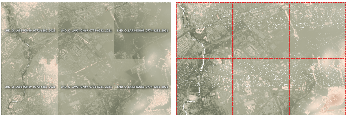
☒ 28.13: Generating Virtual Point Cloud with overview from a set of point cloud tiles
