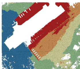
図 28.12: Exporting point cloud (ground points) to a vector layer styled based on the elevation
