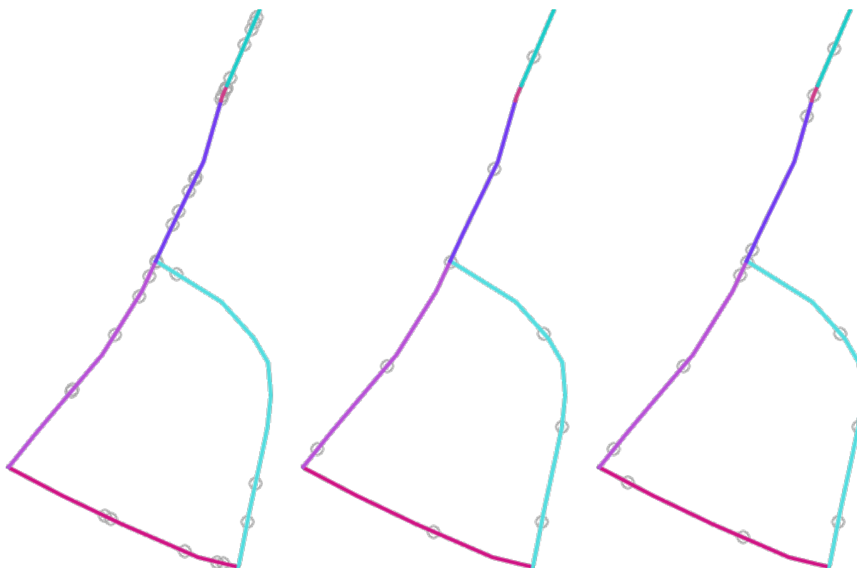
Рис. 28.53: Five points per line feature, left : min. distances = 0, middle : min.distances != 0, right : min. distance != 0, global min. distance = 0
