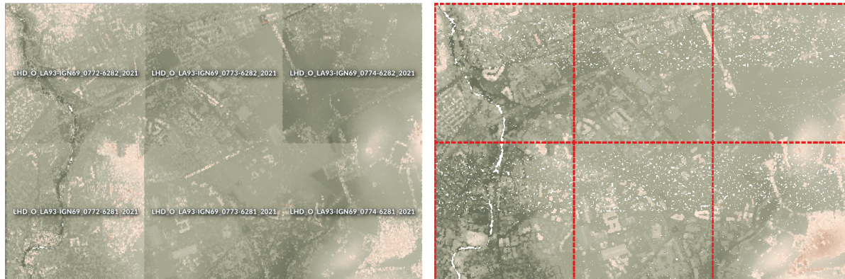
Fig. 28.13: Generating Virtual Point Cloud with overview from a set of point cloud tiles
