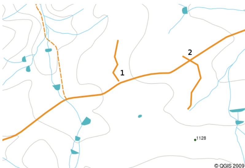
3.13 Fig. : Undershoots (1) occur when digitised vector lines that should connect to each other don't quite touch. Overshoots (2) happen if a line ends beyond the line it should connect to.
