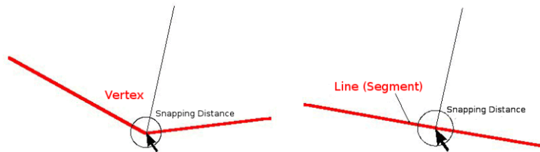
7.4 Fig. : The snapping distance (black circle) is defined in map units (e.g. decimal degrees) for snapping to either vertices or segments.
