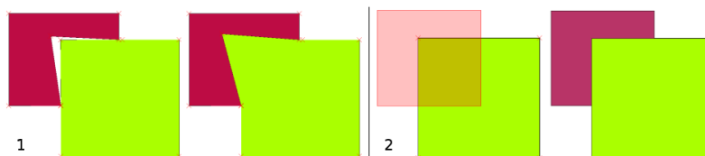
7.3 Fig. : (1) Topological editing to detect shared boundaries, when moving vertices. When moving a vertex, all features that share that vertex are updated. (2) To avoid polygon overlaps, when a new polygon is digitised (shown in red) it is clipped to avoid overlapping neighbouring areas.
