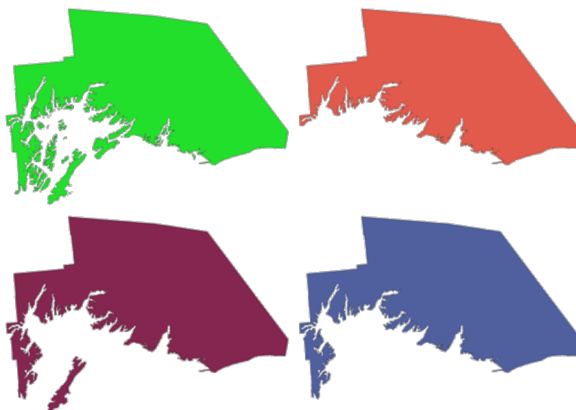
28.88. ábra: Clockwise from top left: original multipart feature, one, two and three biggest parts kept
