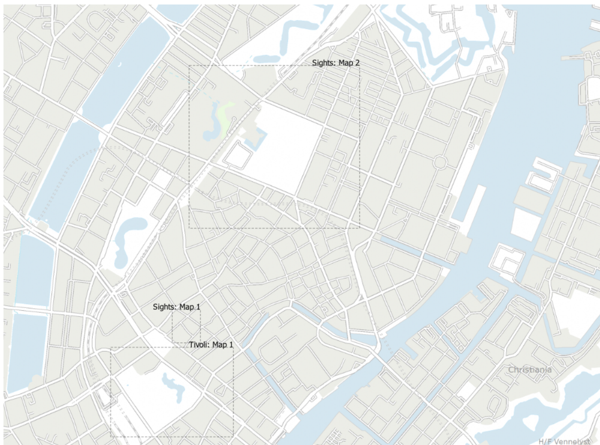
Рис. 11.11: Example of layout extents displayed in a QGIS project with two print layouts. The print layout named „Sights“ contains two map items, while the other print layout contains one map item.
