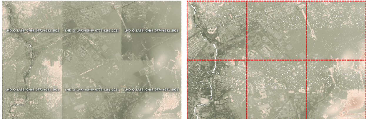
그림 28.13: Generating Virtual Point Cloud with overview from a set of point cloud tiles
