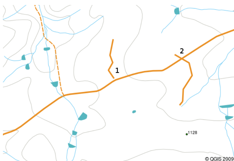
图 3.13: Undershoots (1) occur when digitised vector lines that should connect to each other don't quite touch. Overshoots (2) happen if a line ends beyond the line it should connect to.
